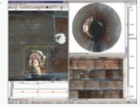
inspection data on one DVD. The new virtual  $360^{\circ}$  pan/tilt view enables the user to select the best sight up to the pipe and gives a virtual review to the crawlers back.
